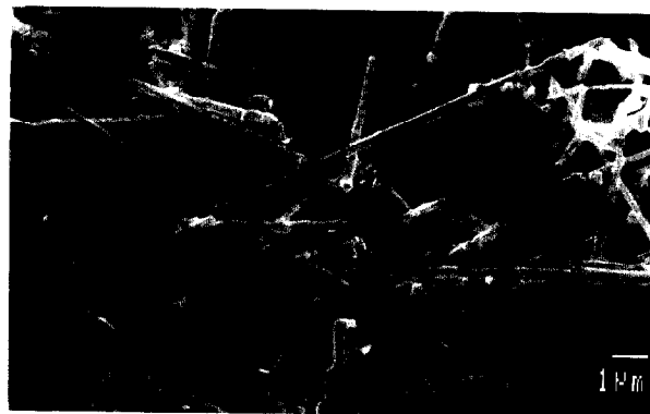
Fig. 1. An SEM micrograph of Ta_{0.5}Ti_{0.5}C whiskers prepared at 1250°C.
